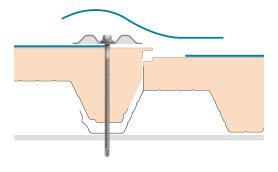
Self-drilling screw; with Metal Plate 82x40mm Type-F and Pontage strip. Number and position of fastenings must be evaluated by Designer.
