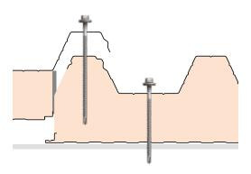
Self-drilling screw; with Ø19mm metal washer. Number and position of fastenings must be evaluated by Designer.
