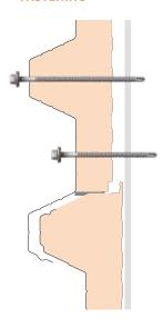
Self-drilling screw; with Ø19mm metal washer.. Number and position of fastenings must be evaluated by Designer.
