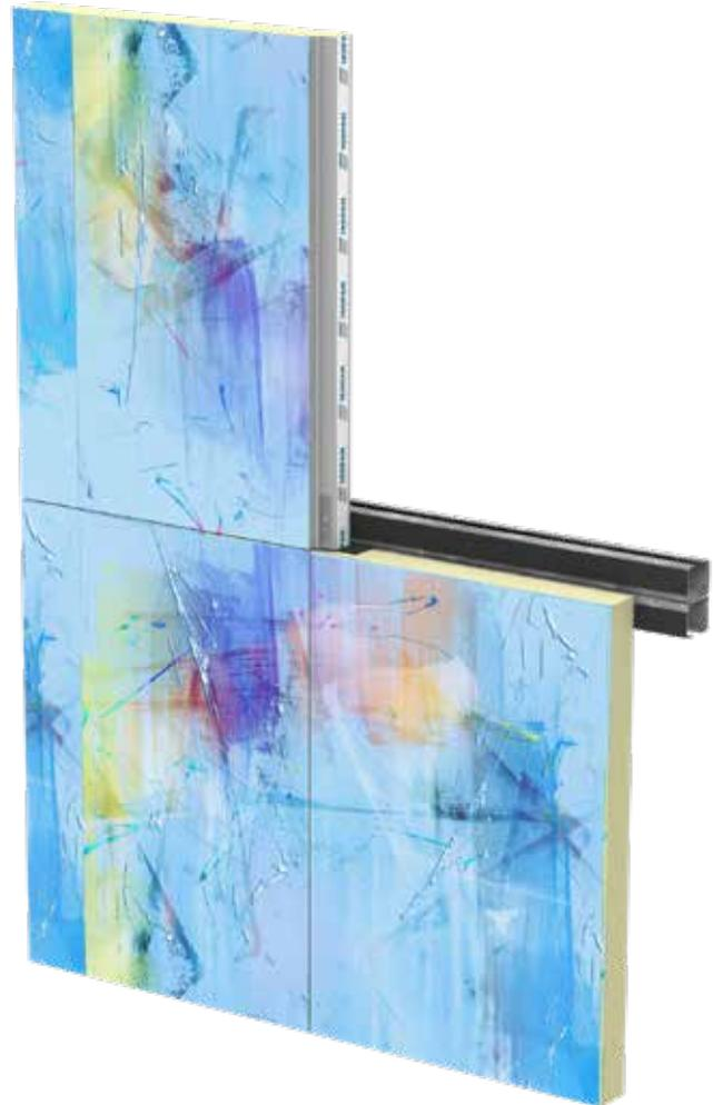
Homogeneous panel made of 30% reinforced thermosetting resins with 70% pressed cellulose fibre in conditions of high pressure and high temperature. Thanks to the innovative technology for surface treatment, the panels feature a surface integrated with the core, compact and decorative, obtained through the use of pigmented polyurethane-based resins. The surface is non porous and easily to clean even in case of acts of vandalism such as graffiti. It does not retain dirt and prevents flaking.
