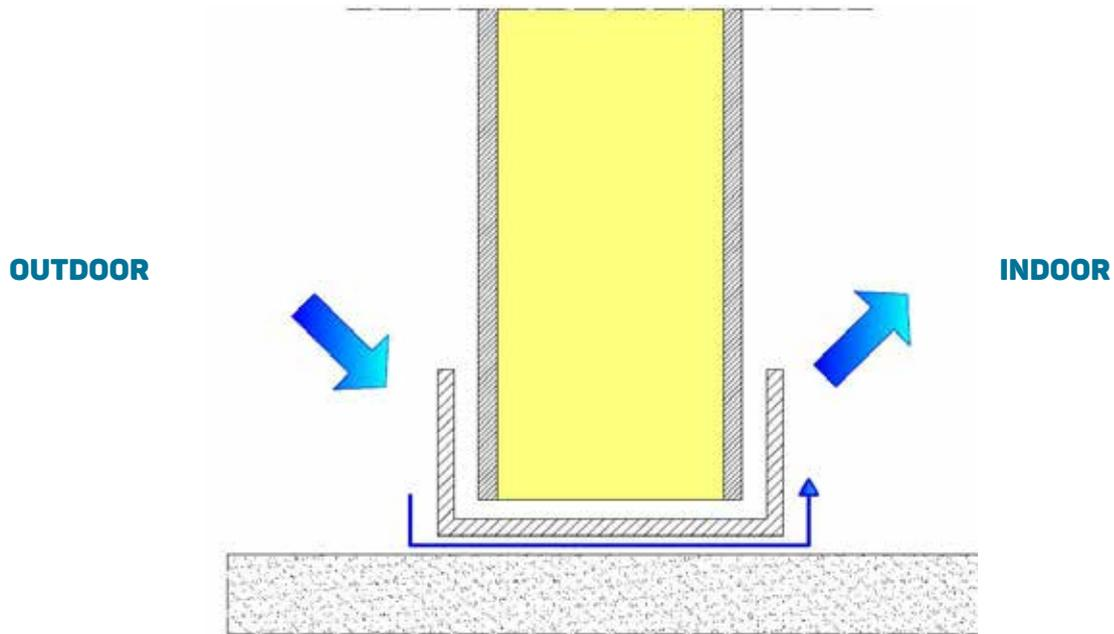
In case of flashing elements the two parts (external and internal surfaces) will have about the same temperature. The internal surface will have a high temperature during the day and a very low temperature at night.
