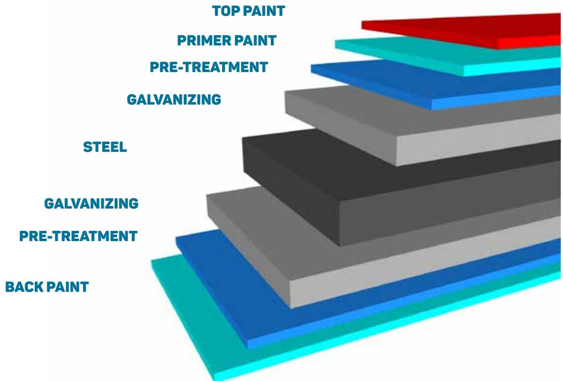
**PAINT LAYERS CAN BE APPLIED WITH ONLY ONE CYCLE OF THE PAINTING LINE BY SIMPLY SETTING THE THICKNESS OF EVERY LAYER.**
